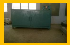
This is a hot air oven is used to cure geo polymer concrete specimens. The capacity of the oven is  $500^{\circ}$ C.
